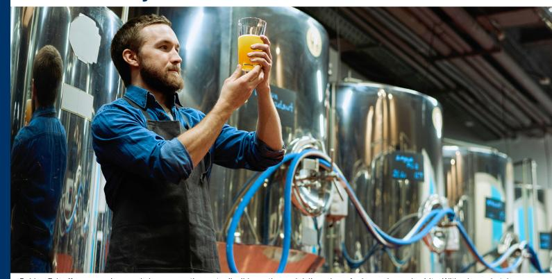
Rubber Fab offers a premium grade low permeation, extra flexible suction and delivery hose for beer, wine and spirits. With a bromobutyl lining, our RFFDABOCCR hose has an improved resistance to higher pressure and is crush resistant.
