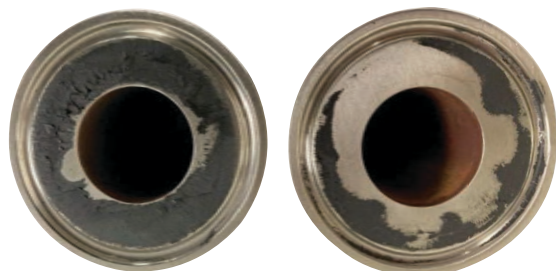
Stainless steel flanges with an EPDM Tri-Clamp ® Gasket adhered to it
