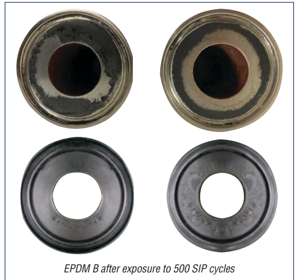
Flex-Pure® after exposure to 500 SIP cycles
